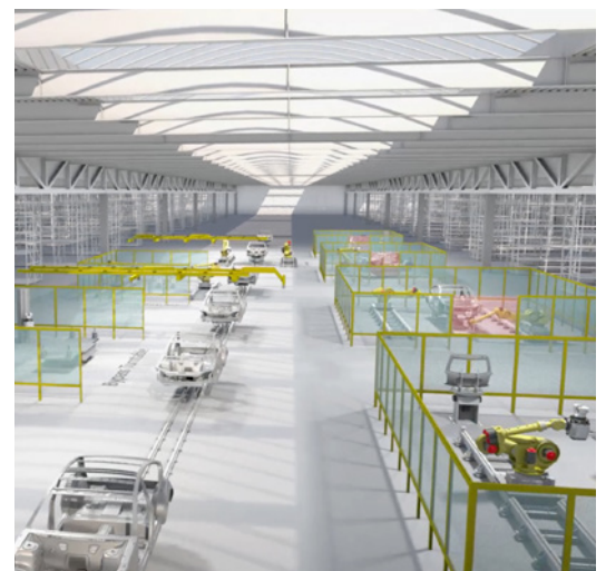
Overview of a automotive shopfloor with bypass, inline and metrology room APDIS installations
